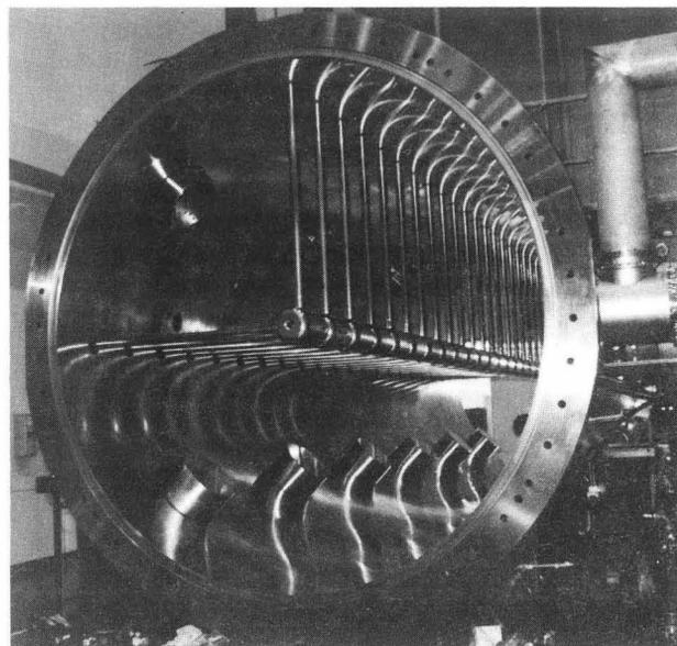
Fig. 1. An inside view of no. 3 Alvarez type linac tank.
