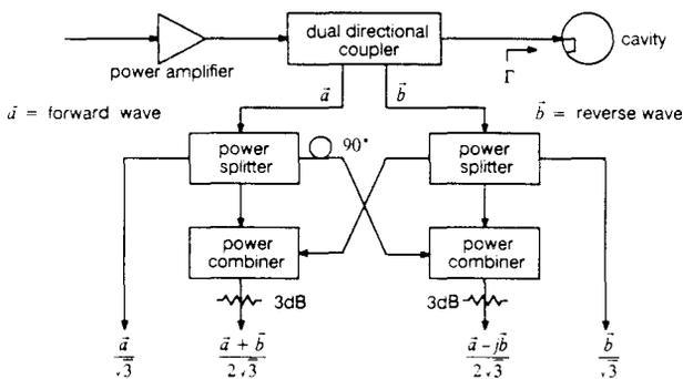
Figure 4. Block diagram of a six-port coupler.
