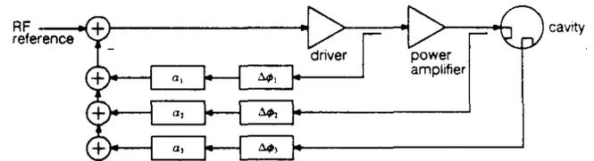
Figure 3. Block diagram of state-variable control system.
