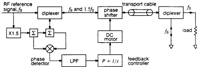
Figure 6. Phase-stable RF transport block diagram.
