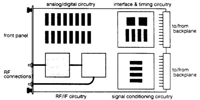
Figure 8. Typical layout of a VXI module for RF control.
