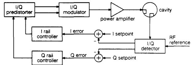
Figure 1. Block diagram of I/Q field control system.
