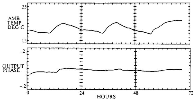
Figure 7. Phase-stable RF transport test results.
