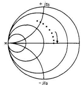
Figure 5. Reflection coefficient locus displayed during resonance control.
