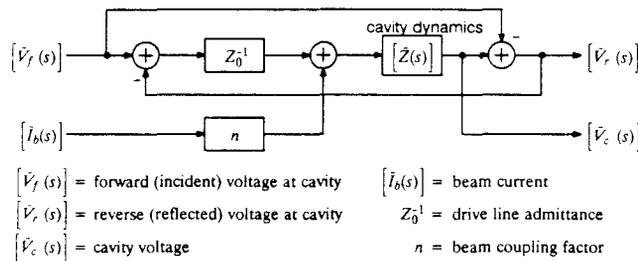
Figure 2. Operational scattering model of a cavity.
