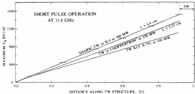
Figure 2. Maximum Surface E-Field Buildup in TW Output Structures.
