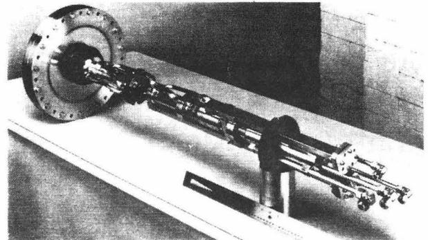
Figure 4. X-791 100MW TW Klystron with Independently Accessible Water Flow Paths for All Five Demountable Sections (Anode, Compression, Gain, Bunching and RF Extraction, and Collector).
