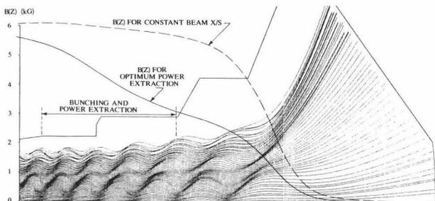
Figure 6. EGUN simulation of DC Beam with Graded Reduction of Axial Magnetic Field over the Output Structure.
