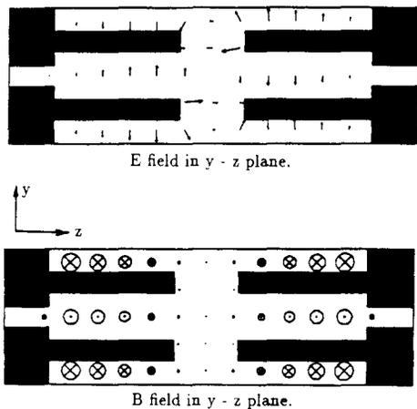
Figure 6. Field patterns in a half-wavelength cavity.
