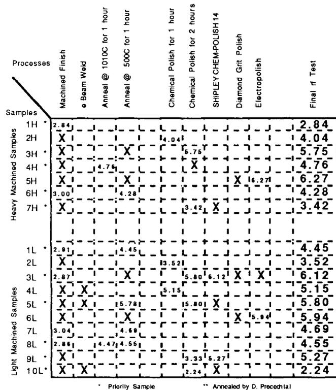
Fig. 1. Q enhancement of the GTA 850 MHz DTL Copper Surface fabrication processes.
