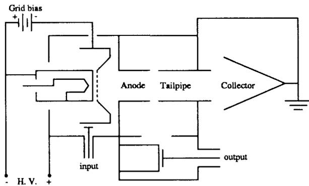
Fig. 1 Schematic of a klystrode with capacitive coupling for both input and output. The klystrode uses a grid to modulate the electron beam density but uses a cavity similarly to a klystron for the output.
