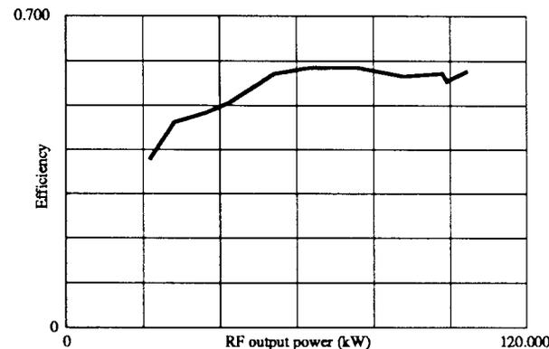
Fig. 5 The efficiency vs input rf power for the klystrode with an anode to cathode voltage of 38kV.
