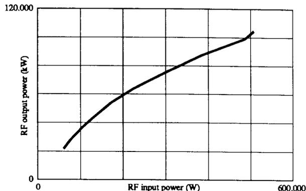
Fig. 3 The output rf power vs input rf power for the klystrode with an anode to cathode voltage of 38kV.
