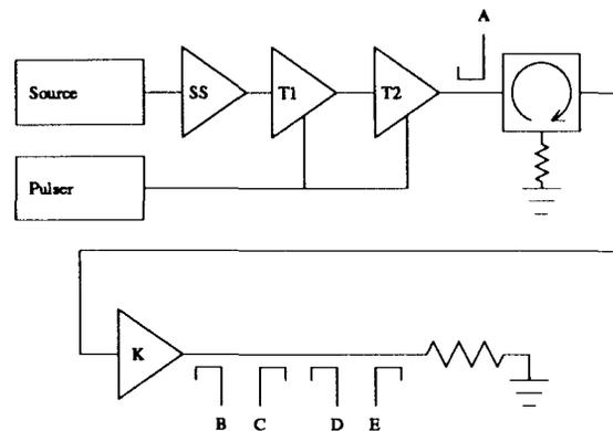
Fig. 2 A schematic of the amplifier chain. The symbols SS, T1, T2, and K respectively correspond to the solid state amplifier, the first triode, the second triode, and the klystrode. The modulation is done by pulsing the grid bias voltage of the triodes. The input to and output from the klystrode, as well as power reflected back to the klystrode, are monitored from the directional couplers labeled A through E. Here a 50Ω load is shown for the output device.
