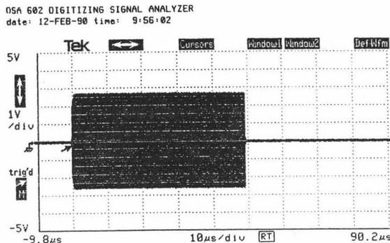
Fig. 6 A typical  $50\mu\text{s}$  long rf pulse at 100kW level.
