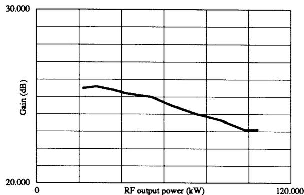
Fig. 4 The gain vs output rf power for the klystrode with an anode to cathode voltage of 38kV.
