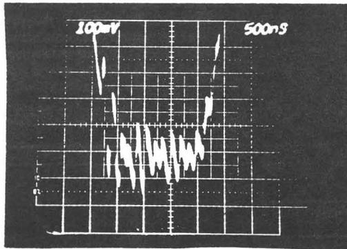
Fig. 6. Expanded pulse top trace of the output pulse current at the dummy load ( $500 \text{ ns}/\text{div}$ ).
