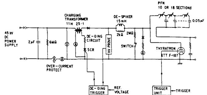
Fig. 3. A simplified diagram of the modulator
