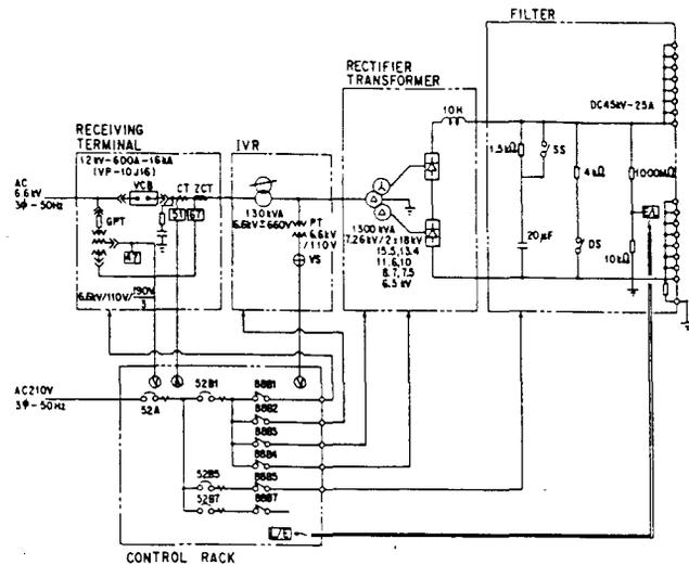
Fig. 2. A simplified diagram of the dc power supply
