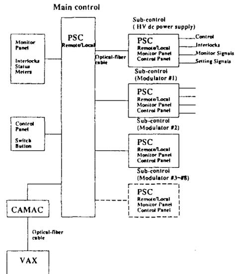
Fig. 4. Block diagram of the modulator control system.
