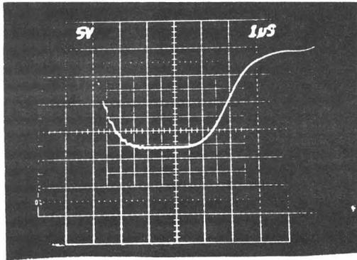
Fig. 5. Output pulse current (peak  $\sim 7200$  A) at dummy load ( $1 \mu\text{s}/\text{div}$ )
