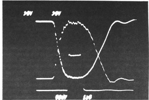
Fig. 7. Output waveform of E3712 klystron at 100 MW
