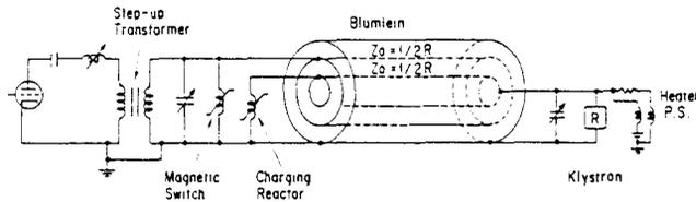
Fig. 4. Simplified diagram of the Blumlein-type modulator.
