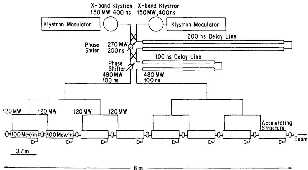
Fig. 1. Conceptual drawing of the JLC microwave distribution system.
