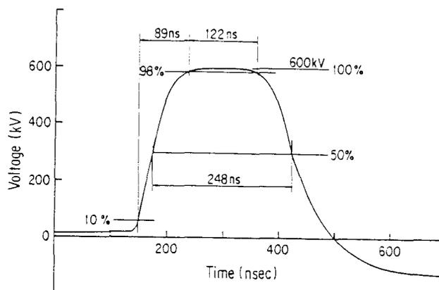
Fig. 3. Simulated output voltage of the X-band klystron modulator.
