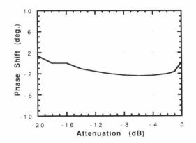
Fig. 5. Phase shift vs. attenuation at 2856 MHz
