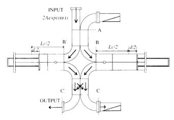
Fig. 2. Attenuator & phase-shifter for the buncher
