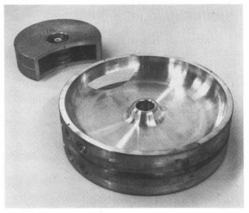
Five Main Cavities and Side Couples were staked on a special fixture and the Pi/2 frequency was measured. One to two additional cuts were needed to achieve the final slot depth. All the remaining cavity sections and bridge ends were machined to this depth.
