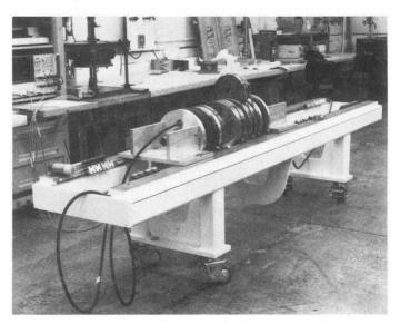
The Bridge Ends, Terminating Ends, and Bridge Side Couples needed special attention. Because of their non-repeating geometry, they require a different frequency than an interior cell. The frequency change was accomplished by removing material from the side wall. The exact frequency was determined when the stack of five is checked for slot depth.
