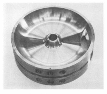
The Main Cavity sections were brought to the tuning lab at Fermilab after machining and each half cell was inspected, labeled, and the frequency measured. From there the Main Cavities went to our machine shop for an initial coupling slot cut.
