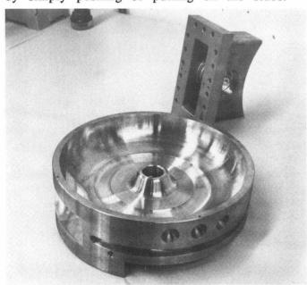
After all the tuning steps are completed in the specially designed stacking fixture, the parts are packed into an air ride cushioned box and shipped by an air ride van to Pyromet Industries in San Carlos, California where they are hydrogen furnace brazed.
