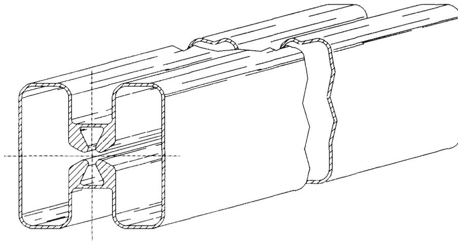
Fig. 2 Conceptual design of a high-frequency SCRFBQ accelerator structure.
