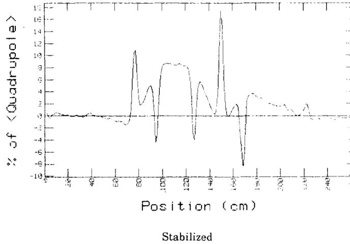
Fig. 7. Dipole perturbation measurements.
