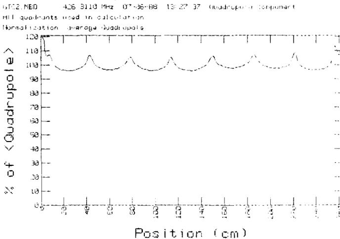
Fig. 8. Quadrupole field with VCRs.
