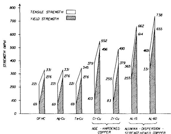
Fig. 1. Tensile and yield strength of coppers.
