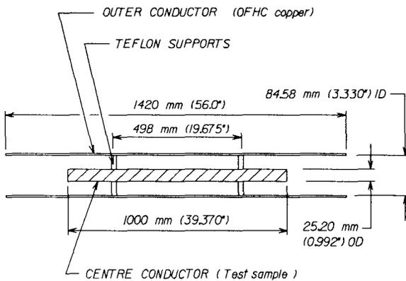
Fig. 3. Resonator structure for the Q measurements
