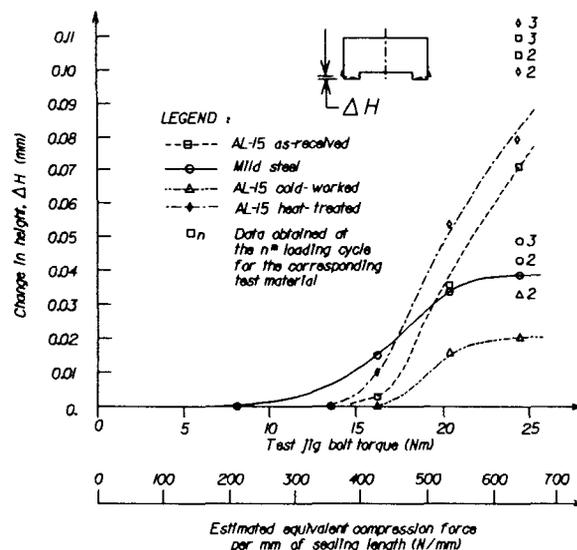
Fig. 2. Change in height of the sealing edges.
