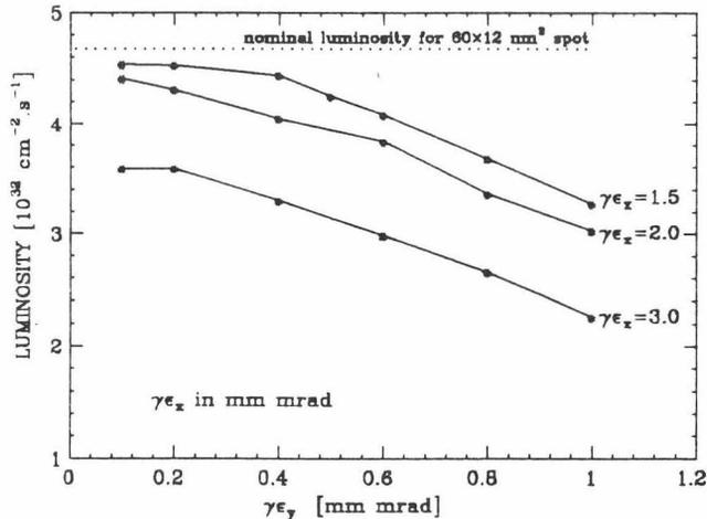
Fig. 10 Luminosity dependence on emittances
