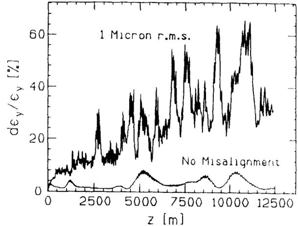
Fig. 5 Vertical blow-up with autophasing
