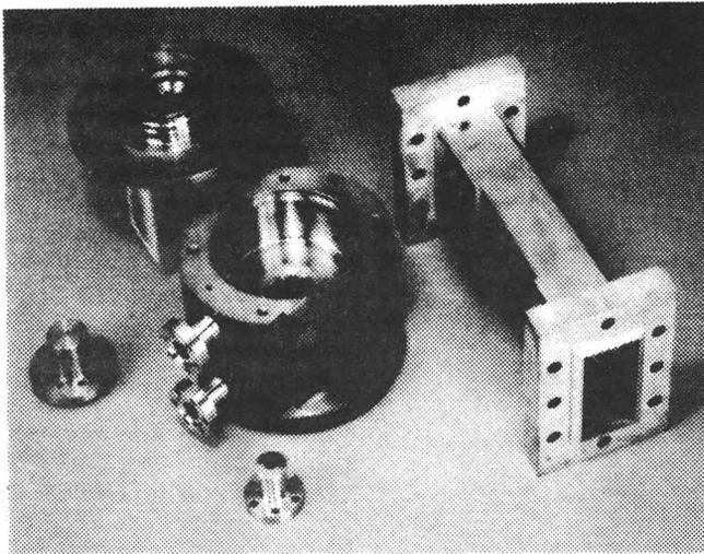
Fig. 2 The test facility RF gun
