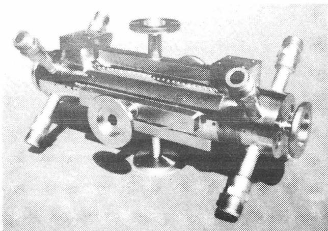
Fig. 7 Finished 30-cell prototype section
