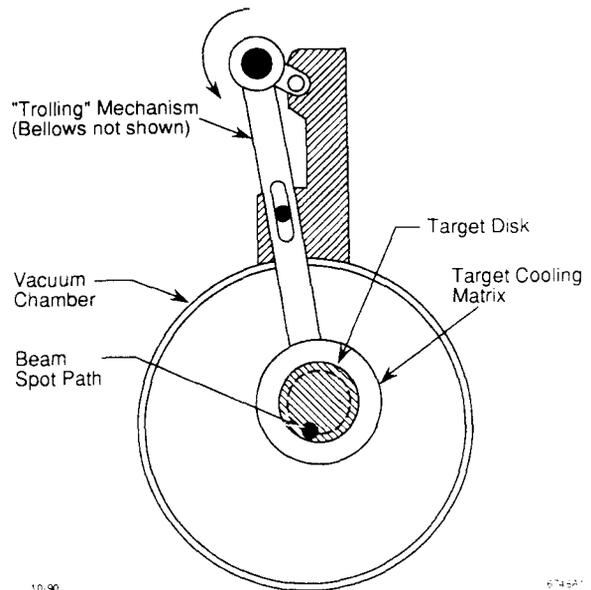
Fig. 4 New high power rotating positron target.
