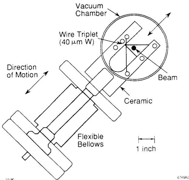
Fig. 6 New wire scanner for the SLC. The wire is made to move through a beam fixed in position.
