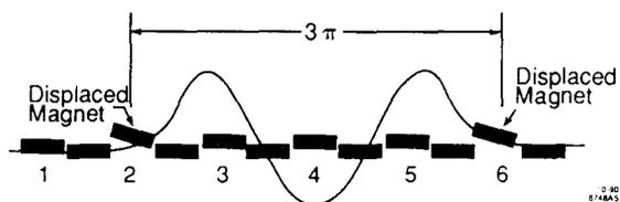
Fig. 12 Magnet 'bumps' in the SLC Arcs which have provided the final needed correction for cross plane coupling.
