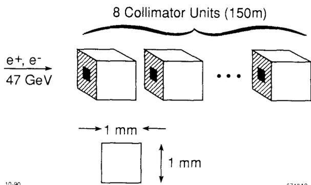
Fig. 13 Adjustable collimators at the end of the linac provide  $3\sigma$  transverse cuts on the beam tails. The eight collimators make a 1 mm square hole over 150 m through which both beams pass. Only 10 to 30 % loss of beam is typical.
