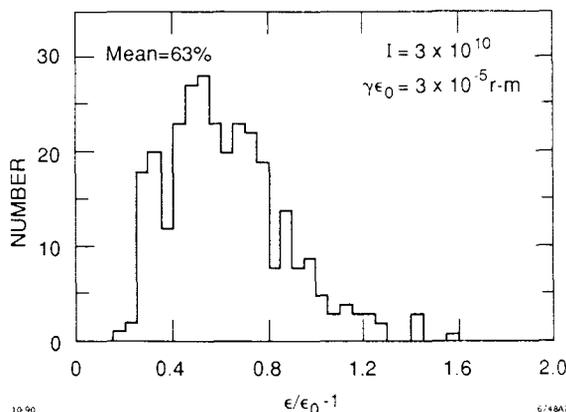
Fig. 9 Emittance growth from accelerator errors for 300 simulated linacs using  $100 \mu\text{m}$  quadrupole and BPM random offsets,  $300 \mu\text{m}$  accelerator errors, 2 % energy scale errors, and 2 degrees input RF phase errors.
