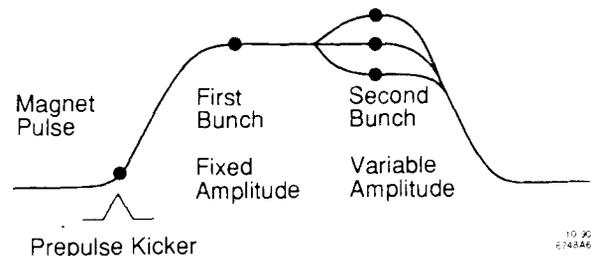
Fig. 5 Improvements to the Damping Ring extraction kicker to allow independent control of both electron bunches.
