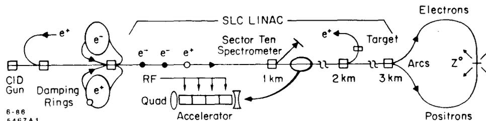
Fig. 1 Schematic view of the Stanford Linear Collider (SLC)
