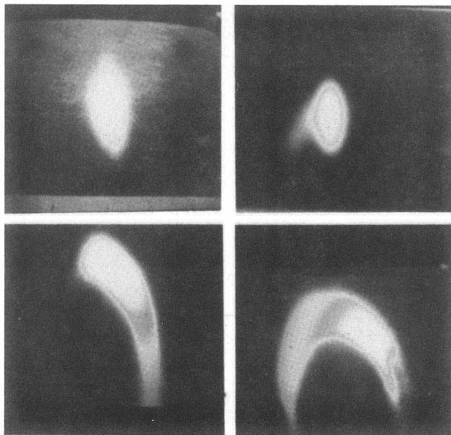
Fig. 10 Observed wakefield beam tails at 47 GeV. The upper left photo shows a well steered beam. The lower right shows a  $3 \times 10^{10}$  e<sup>-</sup> bunch with a 1 mm betatron oscillation.
