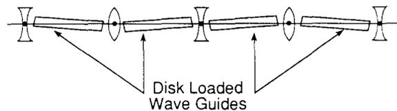
Fig. 8 Schematic view of misaligned accelerating structures.
