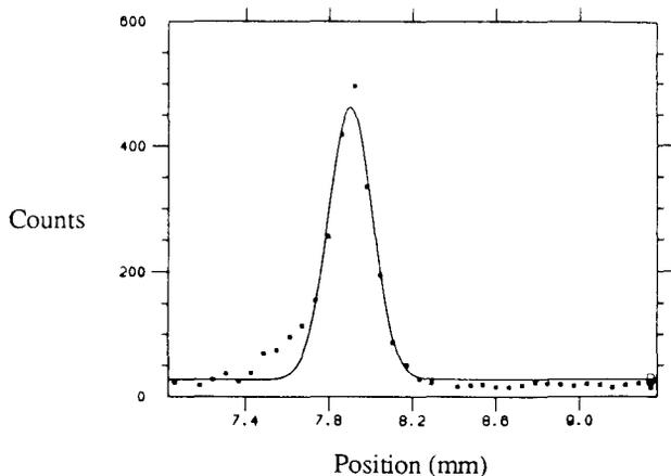
Fig. 7 Measured beam shape showing a wakefield tail. The measured beam size is  $105 \pm 5 \mu\text{m}$ . The invariant emittance is measured using four separated scanners to be  $5. (\pm 0.3) \times 10^{-5} \text{ r-m}$  at  $3 \times 10^{10} \text{ e- / bunch}$ .
