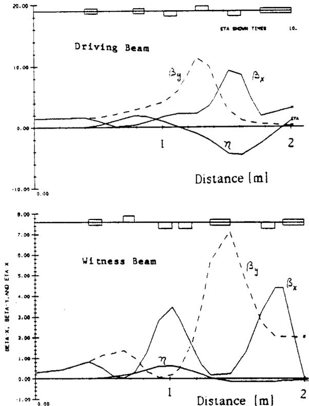
Fig. 2a and 2b. Twiss parameters of beamlines
