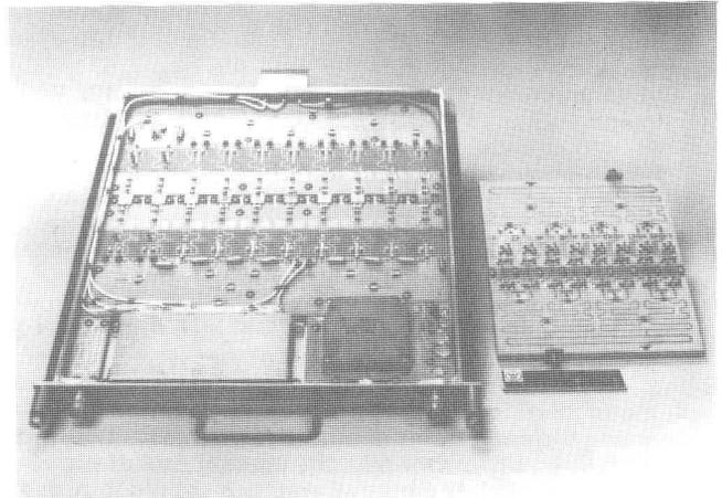
Fig. 1. The 2.5-kW solid-state amplifier modules showing reduction in size using new technology.
