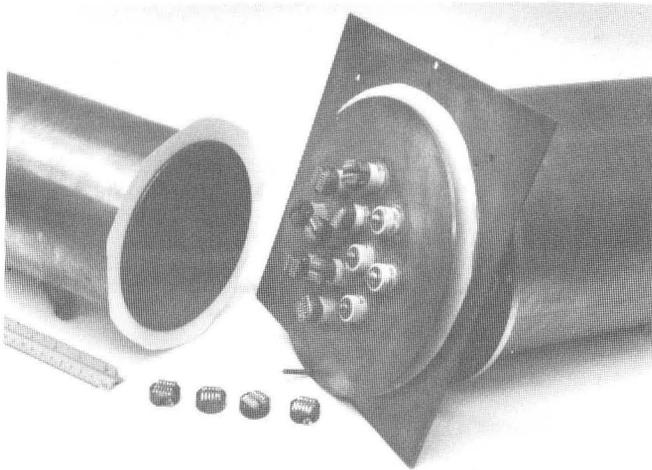
Fig. 5. Multiple planar triode cavity amplifier.
