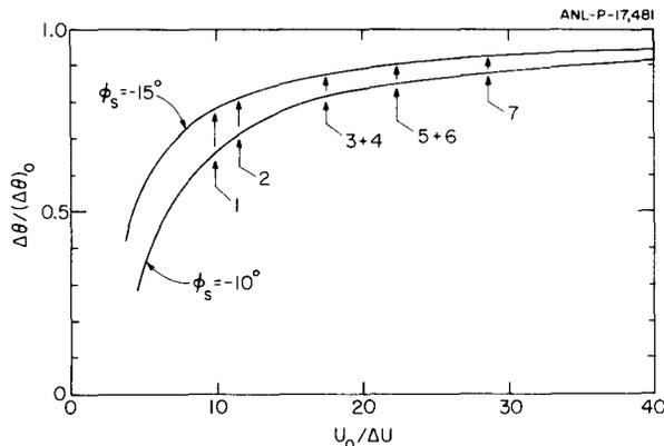
Figure 3. Effects of beam-energy change on radial defocusing angle  $\Delta\theta$ . Values of  $U_0/\Delta U$  for the first seven accelerating resonators are indicated.
