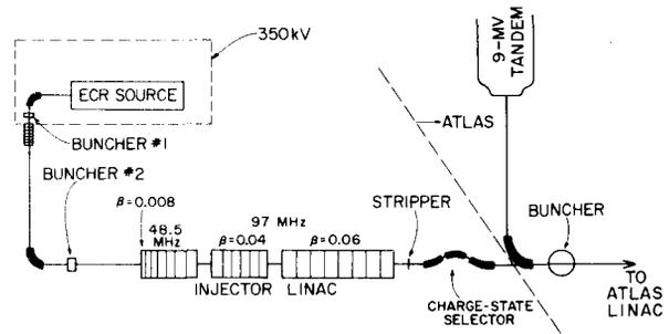
Figure 1. Schematic representation of the proposed heavy-ion injector for the ATLAS linac.
