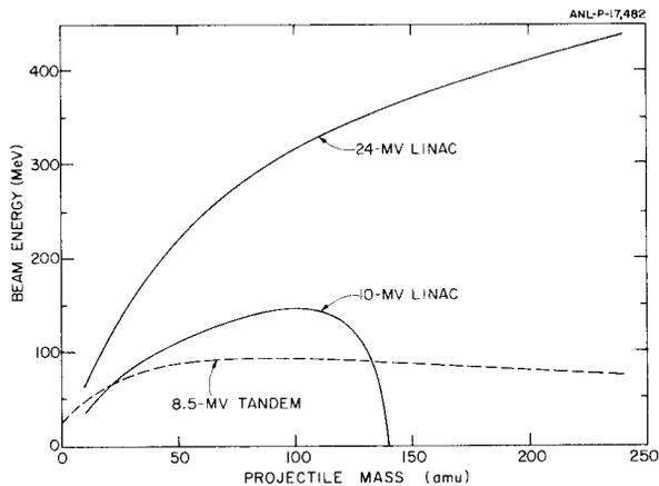
Figure 5. Output beam energy vs mass number for two different configurations of the low-velocity linac.
