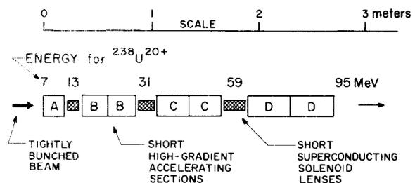
Figure 2. Elements of the very low-velocity superconducting linac. An accelerating gradient of 3 MV/m is assumed.
