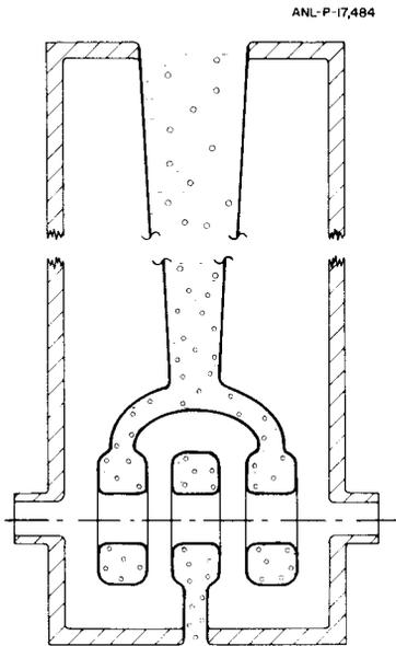
Figure 4. Cross-section of the proposed superconducting niobium resonator. The inductive center-post and forked drift-tube structure are hollow and cooled by boiling of liquid helium.
