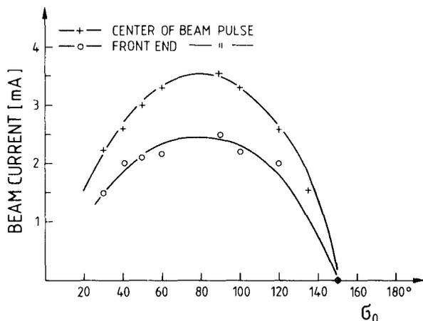
Fig.2: Output current as function of  $\sigma_0$  for the front end and center of beam pulse
