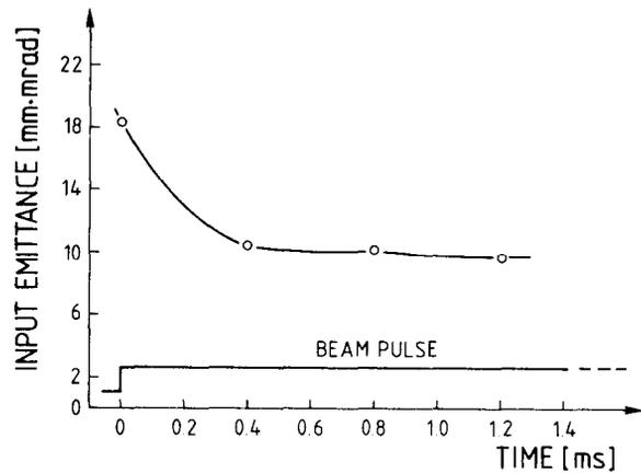
Fig.3: Variation of the beam emittance area along the beam pulse
