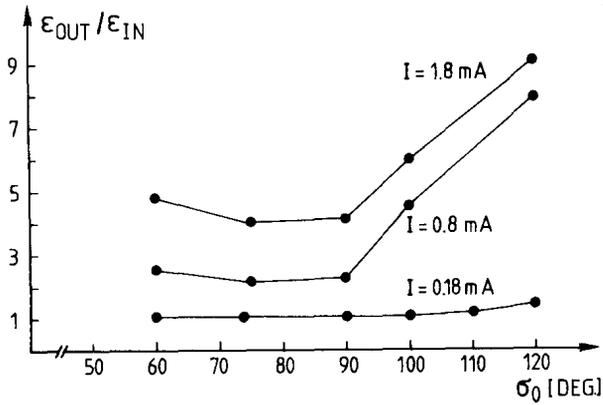
Fig.1: r.m.s. emittance growth versus  $\sigma_0$  for an partially neutralized beam.
