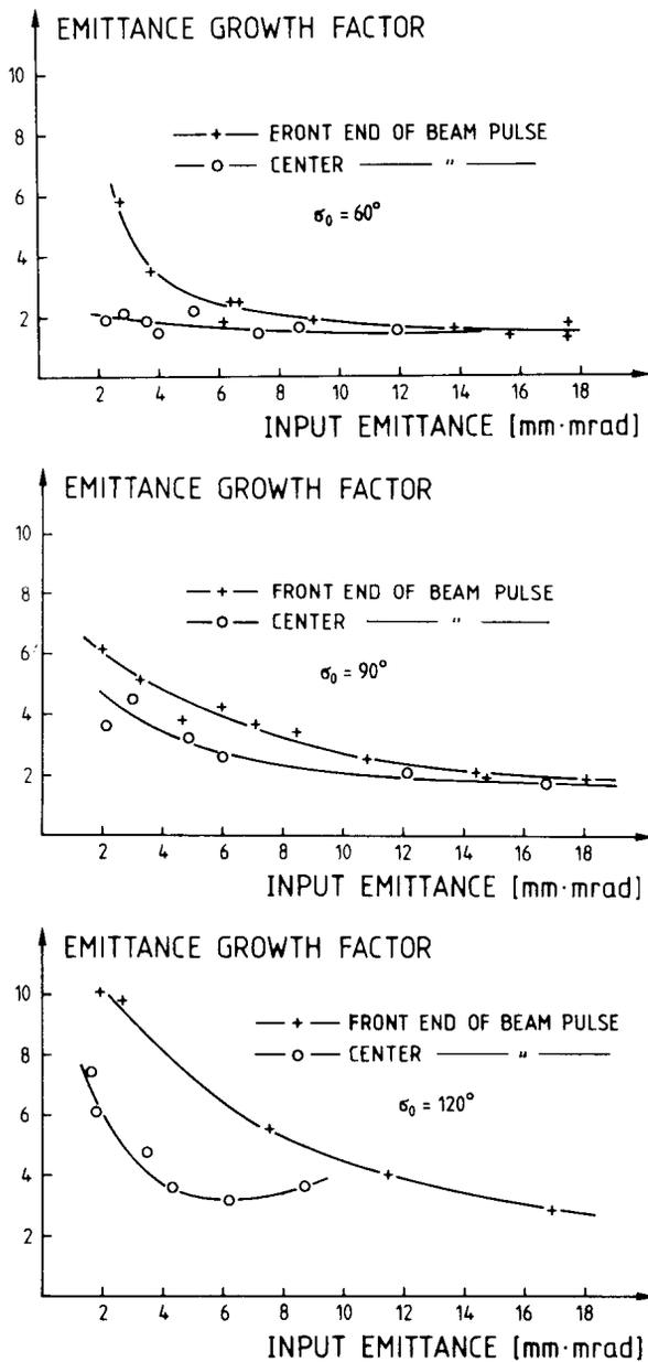
Fig.4: Emittance growth factors for different zero-current tune depressions  $\sigma_0$  and different input emittances.
