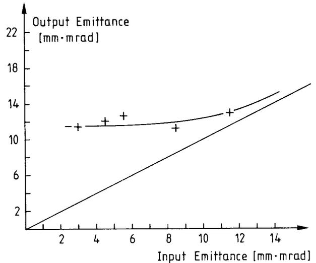
Fig.5: Output emittance versus input emittance after a drift (1m)
