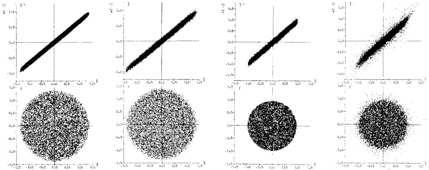
Fig. 3 Intrinsically matched waterbag distribution for periodic focusing with  $\sigma_0 = 60^\circ$ ,  $\sigma = 5^\circ$  at start and after 50 cells.
