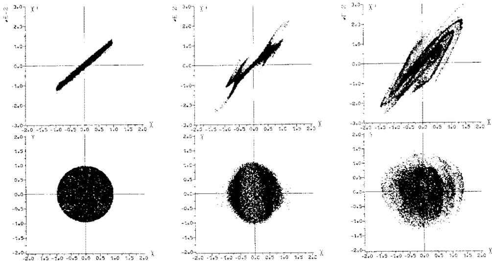
Fig. 2 Instability (of "plasma oscillations") for periodic focusing with  $\sigma_0 = 110^\circ$ ,  $\sigma = 10^\circ$ . Projections into  $x, x'$  and  $x, y$  planes at start ("thermal" distribution with Gaussian velocity distr.) and after 5 and 10 cells.
