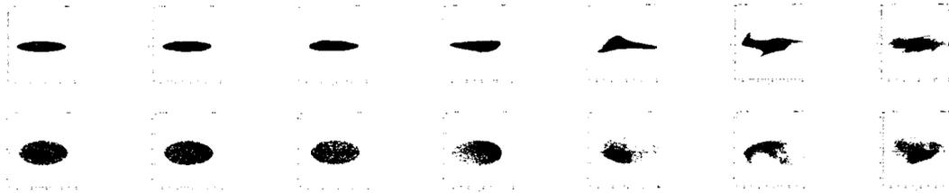
Fig. 1 Third order instability for periodic focusing with  $\sigma_0 = 90^\circ$ ,  $\sigma = 40^\circ$ . Projections into  $x, x'$  plane (upper row) and  $x, y$  plane (lower row) at start (KV-distribution) and in steps of 5 cells.
