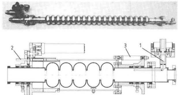
Fig. 3: 20 cell accelerating structure of the Darmstadt s.c. Recyclotron and schematic of a five cell structure including input coupler (1) and tuning system with motor driven course (2) and piezoelectrically driven (3) fine tuner.
