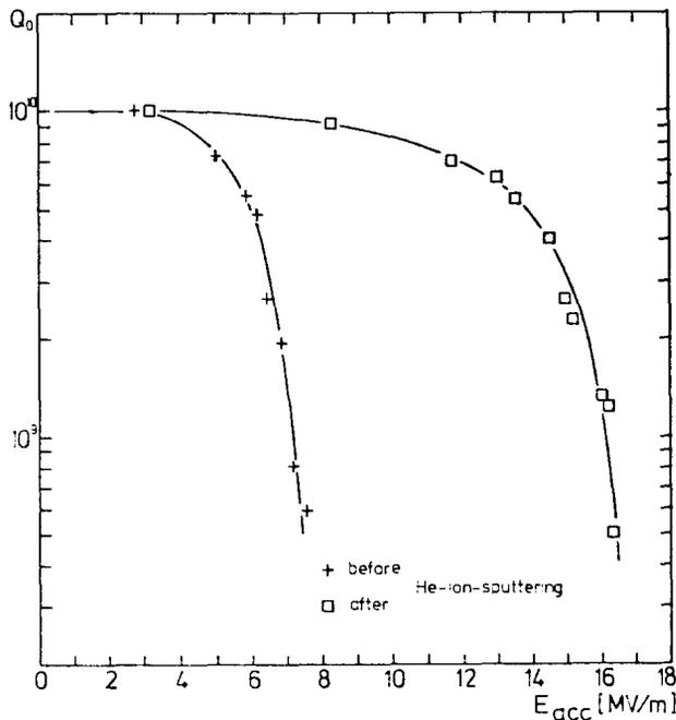
Fig. 8: Dependence of the cavity Q on the accelerating field before and after He-ion sputtering. (T = 1.5 K)
