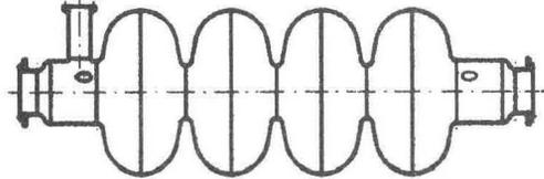
Fig. 2: Design of the new s.c. prototype resonator for LEP
