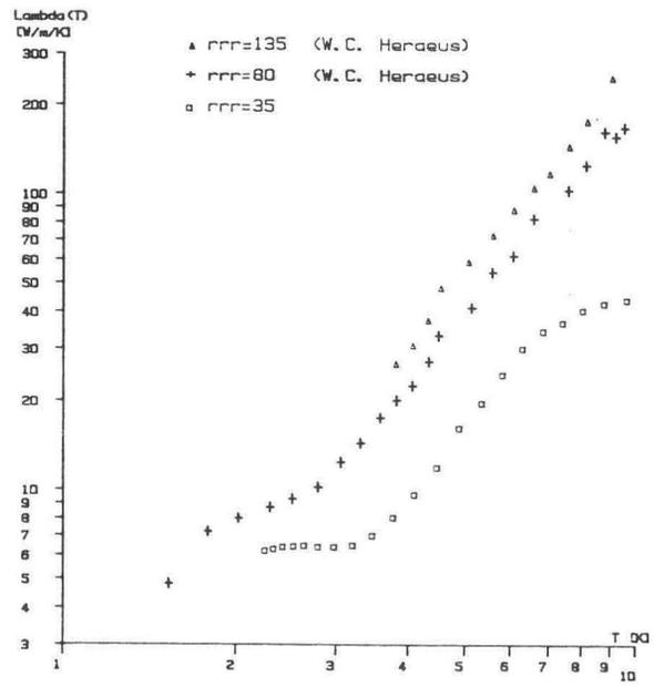
Fig. 5: Temperature dependence of the thermal conductivity of niobium sheet material of different Residual Resistivity Ratios (RRR).
