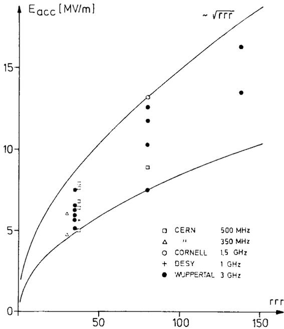
Fig. 6: Dependence of the quench field of different single cell cavities and their thermal conductivity.
