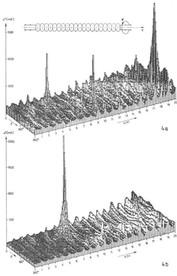
Fig. 4: Temperature map of the 20 cell accelerating unit of the Darmstadt Recyclotron after first test (fig. 4a, quench field 3.7 MV/m) and after grinding (fig. 4b, quench field 4.2 MV/m, showing the creation of a new defect during the repair cycle. The coordinate S(Z) measures the surface distance along the axial direction Z of the structure. The temperature elevation ( $\Delta T$ ) in the iris regions is due to the reduced cooling of these zones in the subcooled helium bath.
