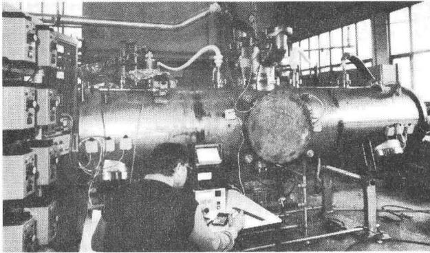
Fig. 1: DESY cryostat housing two nine cell (1 GHz) accelerating structures.
