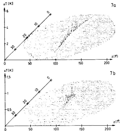
Fig. 7: Two temperature maps of the CERN 500 MHz cavity. Fig. 7a shows the temperature increase induced by electrons emitted from single source. Fig. 7b shows the cavity during quenching initiated by field emission. The temperature increase  $\Delta T$  of the outer surface of the cavity is plotted against the surface coordinates  $s(Z)$  and  $S(\phi)$ .  $S(Z)$  is the length (in arbitrary units) measured along the meridian of the cavity surface and  $S(\phi)$  gives the azimuthal location.
