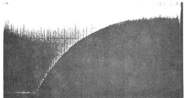
Fig. 5. Decay of oscillator power at end of macropulse provides a measurement of resonator losses.
