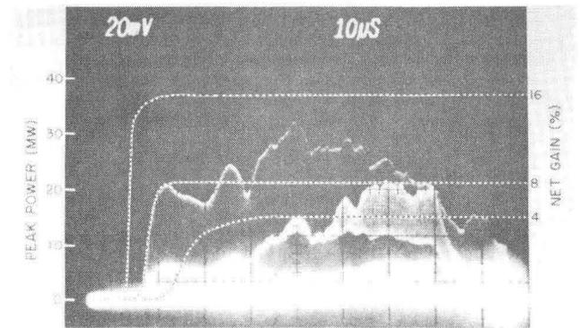
Fig. 4. Optical power within Los Alamos FEL oscillator during one macropulse.
