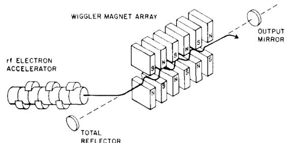
Fig. 1. The basic elements of a Compton-regime FEL oscillator: relativistic electron beam, magnetic wiggler, and optical resonator.
