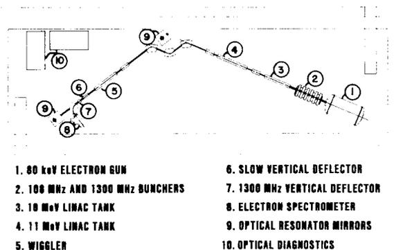
Fig. 2. Layout of Los Alamos FEL oscillator experiment.
