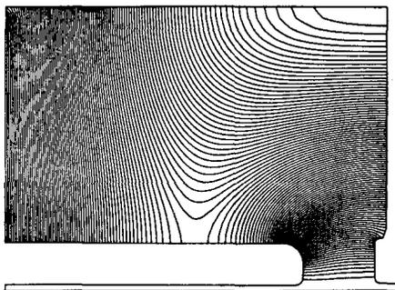
Fig. 1. One-quarter cross section of dummy drift-tube tank showing electric field lines.
