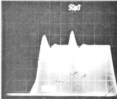
Fig. 7. Vertically expanded cavity rf field (total peak-to-peak voltage = 18 V) (500 mV, 50 µs/DIV).
