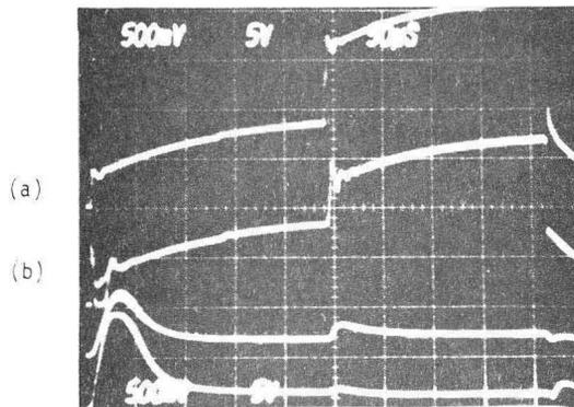
Fig. 4. (a) Master chain forward power (open loop). (b) Slave chain forward power (closed loop). (100 kW/DIV, 50 μs/DIV)
