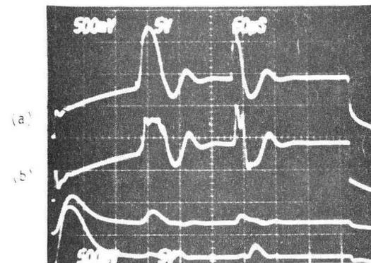
Fig. 5. (a) Master chain forward power (closed loop). (b) Slave chain forward power (closed loop).
