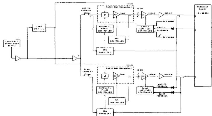
Fig. 2. Simplified schematic for rf control-system experiments.
