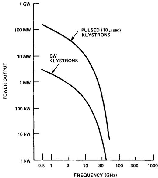
Fig. 1. Technology Limits for Pulsed and CW Klystrons.
