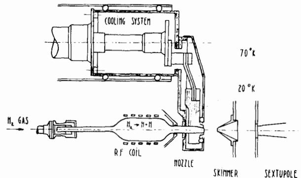
Fig. 2 : the nozzle cooling system
