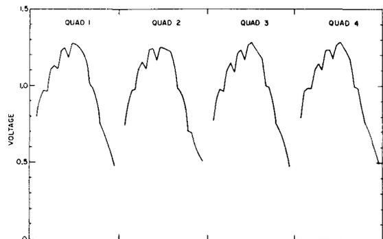
Fig. 1. A magnetic perturbation measurement of RFQ2 with seven VCR pairs located at the λ/2 points of the structure.
