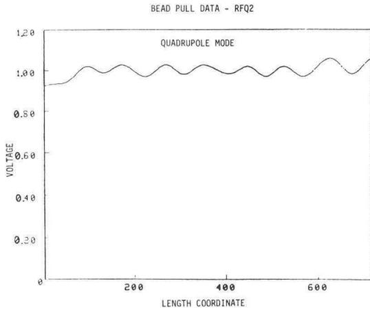
Fig. 5. Longitudinal variation of the quadrupole field shown in fig. 5 after adjusting end tuners.
