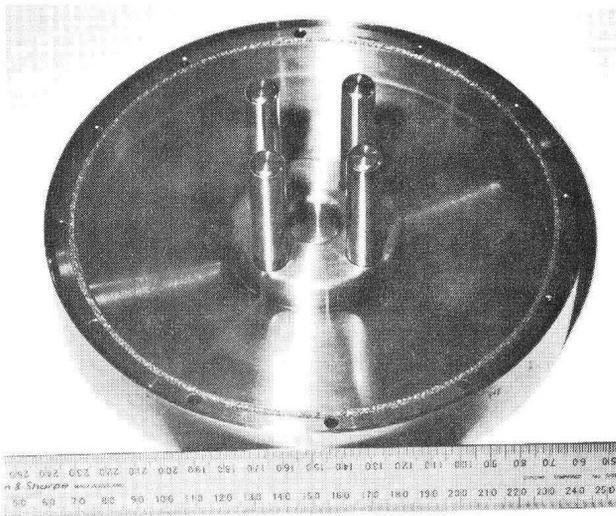
Fig. 6. End tuners used in RFQ2. The tuning stubs insert into the quadrants rather than face the vane ends.
