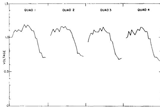
Fig. 3. Quadrant voltage distributions with seven alternating horizontal and vertical VCRs located at the  $\lambda/2$  points. Vane extenders located at the output end of the vanes have been used to raise the field at the input end for this preliminary measurement.
