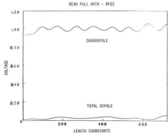
Fig. 7. Quadrupole and dipole components of the RFQ field from the final tuning measurements.
