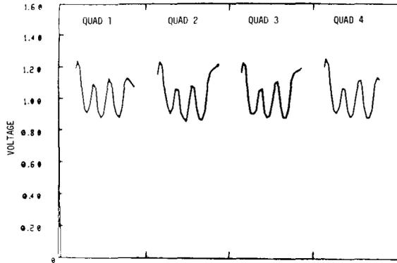
Fig. 2. Magnetic perturbation measurements of the RFQ with four VCR pairs.
