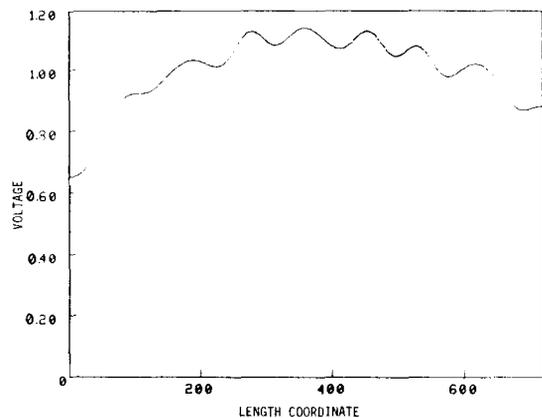
Fig. 4. Longitudinal variation of the quadrupole field after vane shimming and ring adjustment. Data for this measurement were taken with an on-axis dielectric bead pull.
