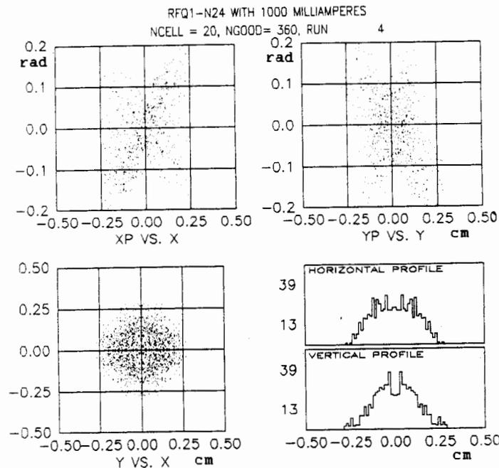
Fig. 3 Particle distribution at output plane of cell 20, with 1000 milliamperes beam current.
