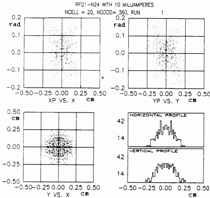
Fig. 2 Particle distribution at output plane of cell 20, with 10 milliamperes beam current.
