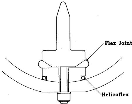
Fig. 1 RFQ1-A vane mounting detail.
