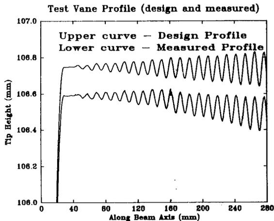
Fig. 4 Test vane profile.
