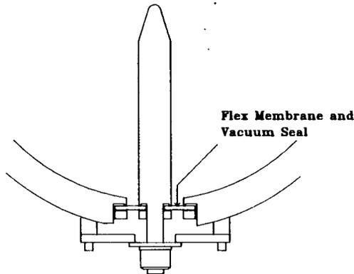
Fig. 2 RFQ1-B vane mounting detail.
