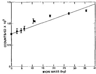
Fig. 6. Gross gamma ray counts per number of coulombs of collected charge due to added iron as determined from 7631.13- and 7645.45-keV lines.
