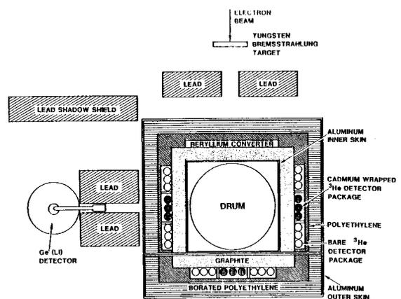
Fig. 1. Experimental arrangement showing 208-liter barrel counter and the Ge(Li) detector with its shielding.
