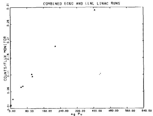
Fig. 4. Response of barrel counter versus mass of  $^{239}\text{Pu}$  placed in center of counter. Combined EG&G/EM/DOE and LLNL linac runs.
