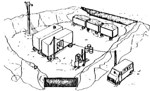
Fig. 7. Artist's conception of electron-accelerator-based mobile assay system for TRU waste. The linac, barrel counter with gamma capture spectrometer, and control and data acquisition system are housed in trucks or truck trailers. Necessary shielding is built on site from available materials.
