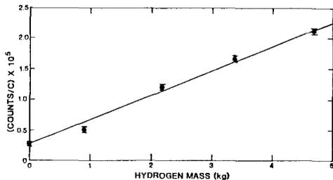
Fig. 5. Gross gamma ray counts per number of coulombs of collected charge due to added hydrogen as determined from 2223.25-keV line.
