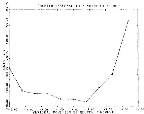
Fig. 3. Response of barrel counter to a point  $^{252}\text{Cf}$  neutron source.
