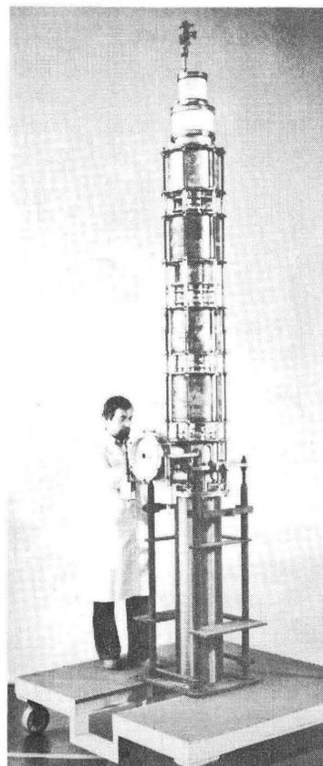
1,5 MW Klystron V107SK
