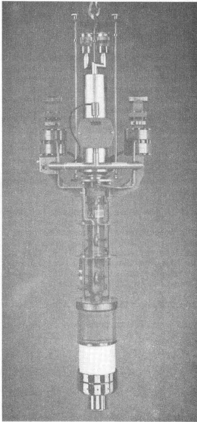
35 MW Pulse-Klystron YK 1600
