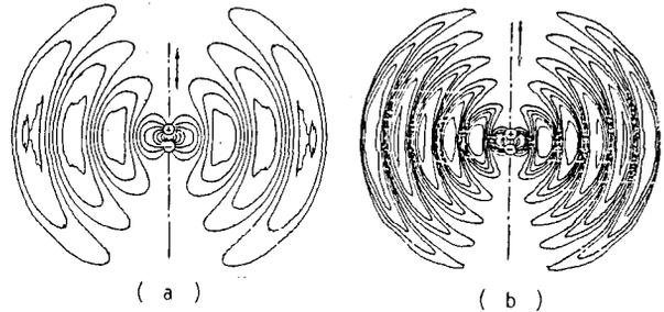
Fig. 7. The electric field pattern of the dipole radiation. The maximum velocity of the oscillation is ( a )  $\beta_{max} = 0.5$ , ( b )  $\beta_{max} = 0.8$ .
