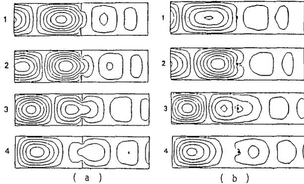
Fig. 5. Propagation of microwave in a rectangular wave guide with ( a ) an iris, ( b ) a rod. The right end line is the free boundary. The mesh size is 10 x 40.
