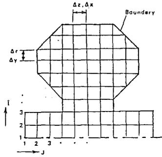
Fig. 3. The rectangular mesh for the finite difference method.
