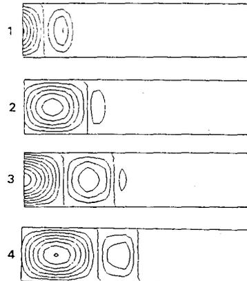
Fig. 4. The propagation of the pulsed microwave. The mesh size is 10 x 40. The width of the wave guide is 10 cm and the frequency is 2600 MHz.
