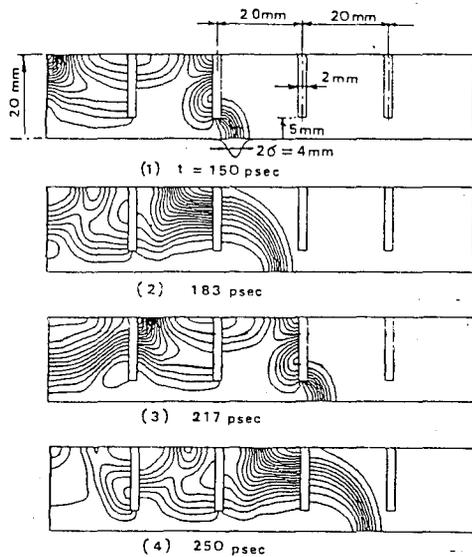
Fig. 6. Beam induced field in a disk loaded accelerating structure. The mesh size is 20 x 100.
