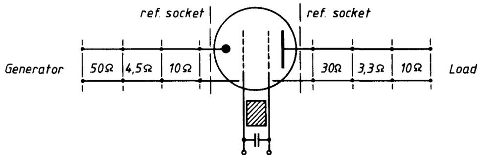
Fig. 2 Equivalent circuit of the amplifier
