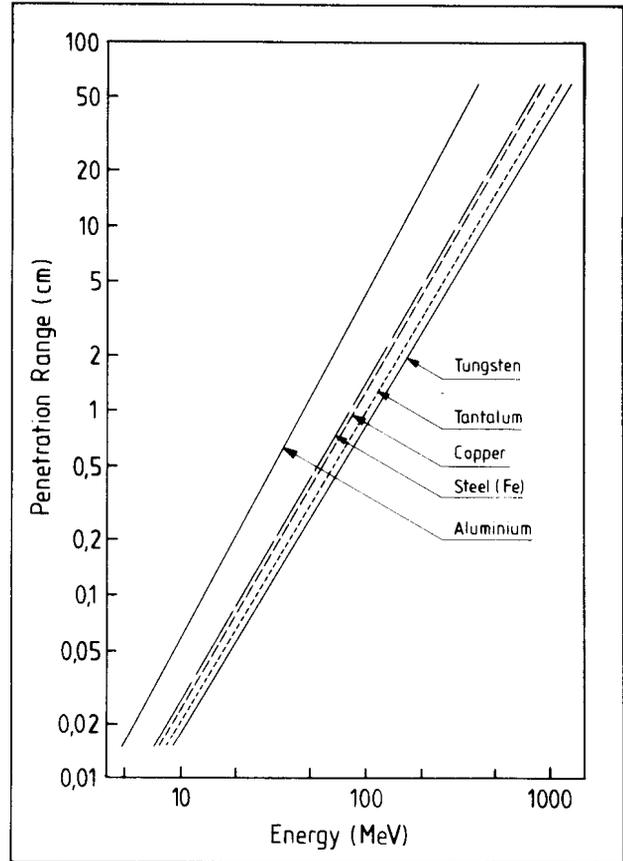
Fig. 4: Penetration range of protons for various materials vs. proton energy
