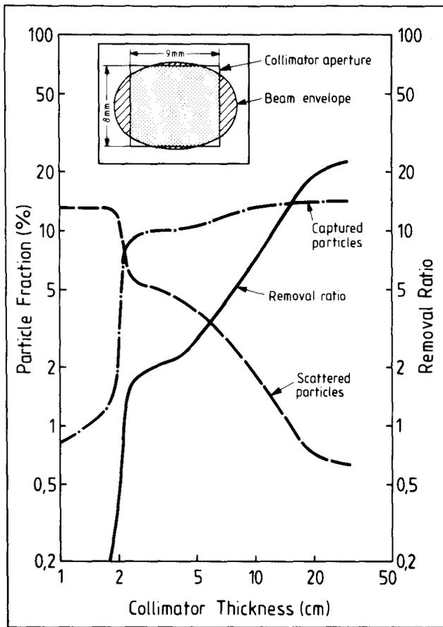
Fig. 1: Removal ratio and particle fractions vs. collimator length for a copper collimator positioned at a proton energy of 100 MeV
