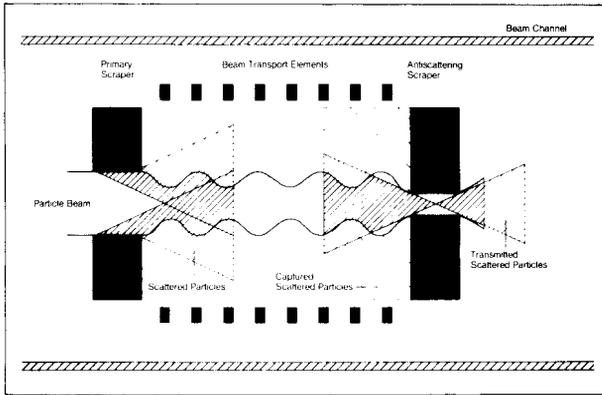
Fig. 3: Schematic representation of the generation and removal of scattered particles in a collimator doublet
