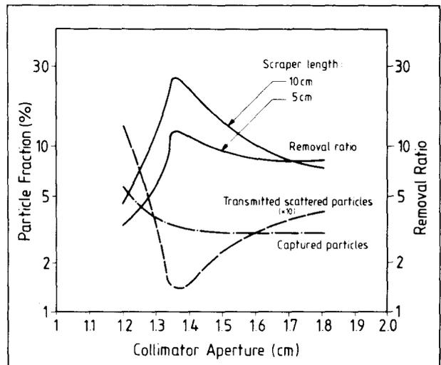
Fig. 2: Removal ratio and particle fractions behind a collimator doublet vs. secondary collimator aperture for a proton energy of 100 MeV
