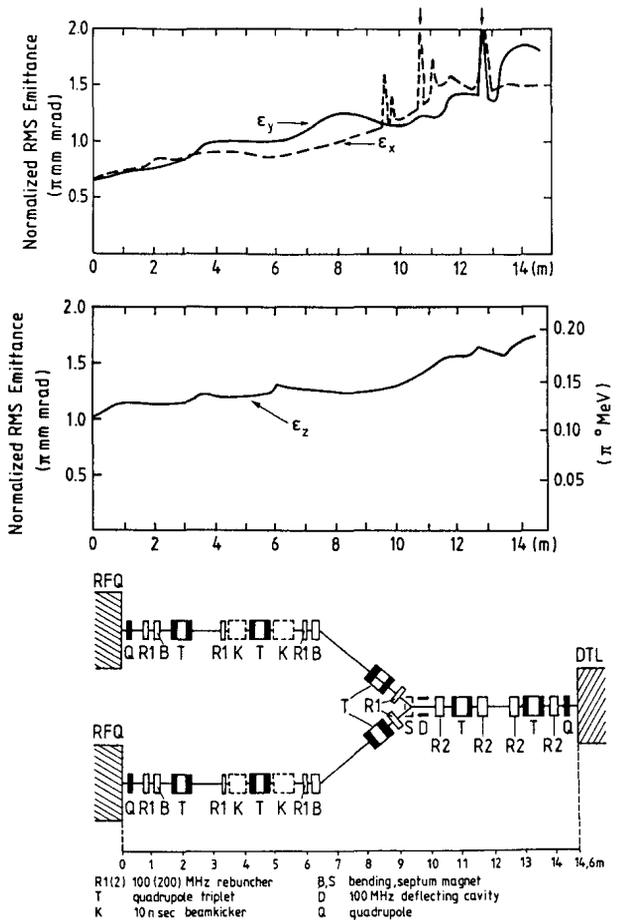
Fig. 2: rms emittances along the funneling line
