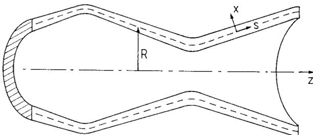
Fig. 1 The beam envelope in a strong focusing channel for hollow beams is modulated. All the forces are calculated with respect to a reference trajectory surface, shown as a dashed line.
