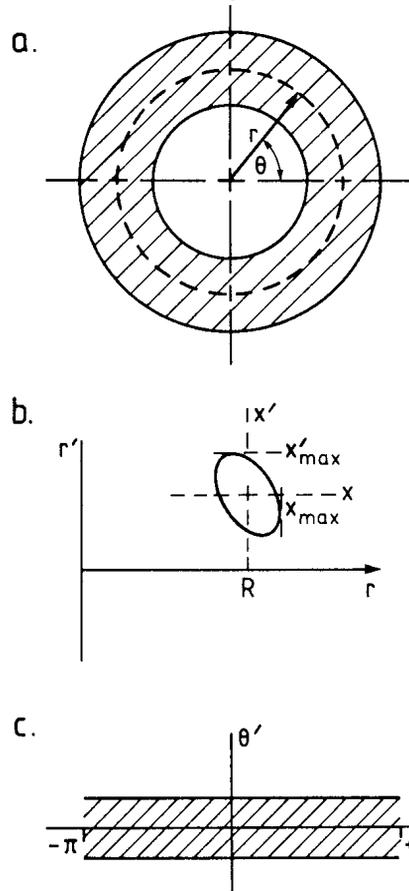
Fig. 2: Emittance definition for hollow beams
