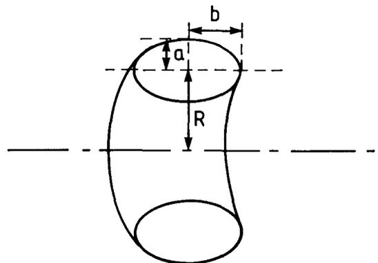
Fig. 3 Space charge forces in a bunched hollow beam are analysed by considering the charge to be uniformly distributed inside a toroid having an elliptical cross-section.
