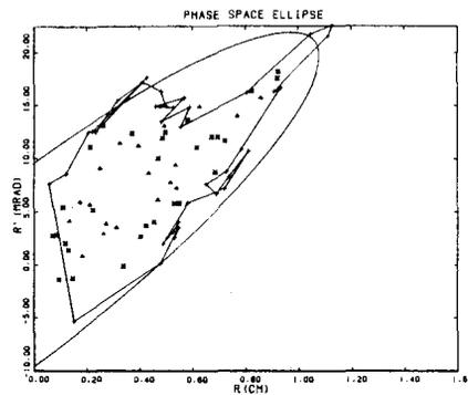
Fig. 3. Beam drifted 70 cm at 3.0 MeV and 500 A with emittance of 10.33 cm-mrad.
