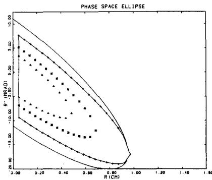
Fig. 1. Initial convergent beam with emittance of 10.01 cm-mrad. Three sets of rays are designated by different markers.
