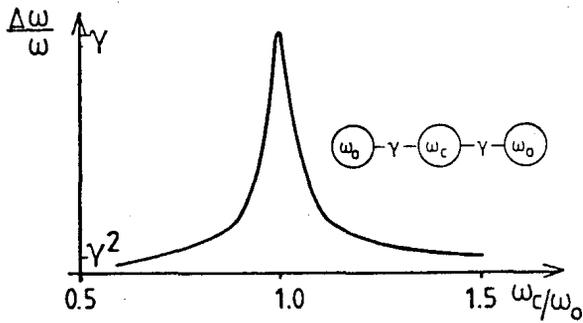
Fig. 3 Coupling strength as function of coupling cell frequency
