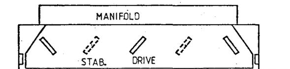
Fig. 11 Manifold as stabilizing coaxial line
