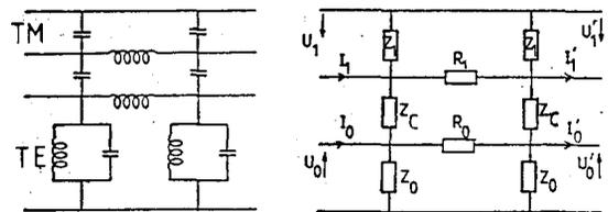
Fig. 10 TE-stabilization network
