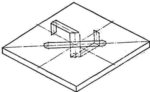
Fig. 5 Sketch of orthogonal loop in a coupling slot
