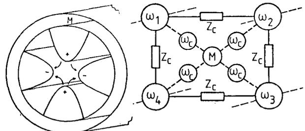
Fig. 1 Scheme of an RFQ resonator system
