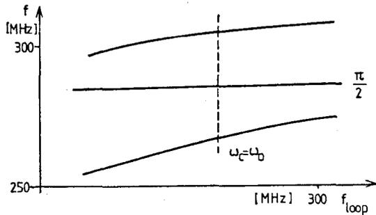
Fig. 4 Mode frequencies of loop coupled coaxial resonators
