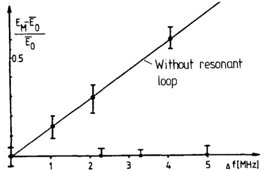
Fig. 7 Field tilt versus detuning frequency
