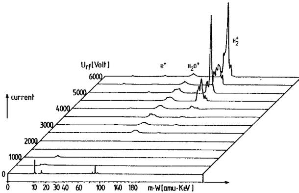
Fig. 4 Energy spectrum behind section 4 of the proton model
