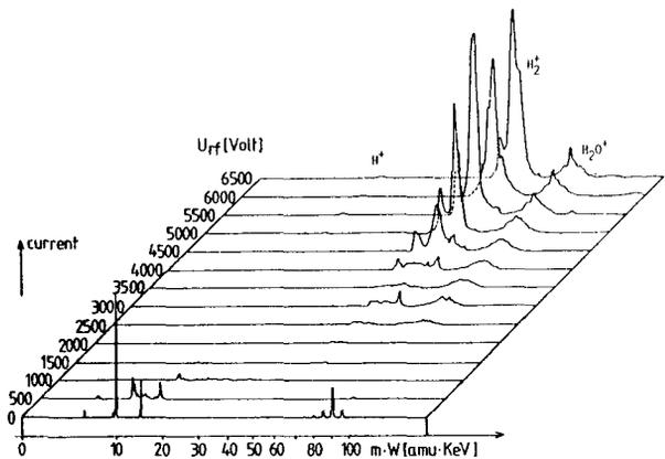
Fig. 2 Energy spectrum behind section 2 of the proton model
