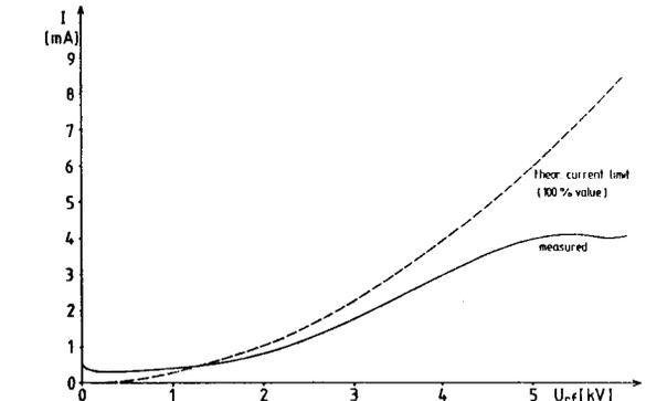
Fig. 11 SCR beam transport: Theoretical current limit and experimental result as a function of RF voltage
