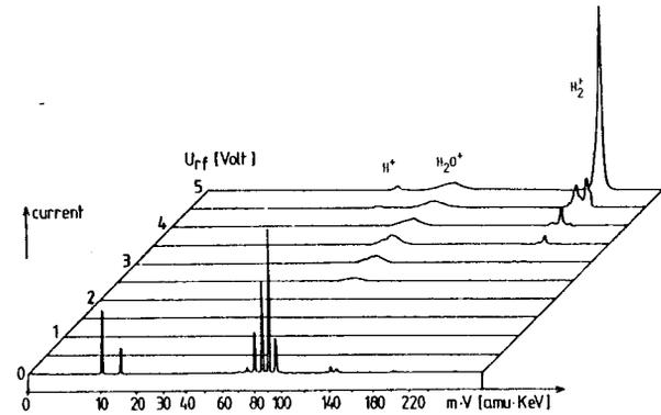
Fig. 5 Energy spectrum behind section 5 of the proton model
