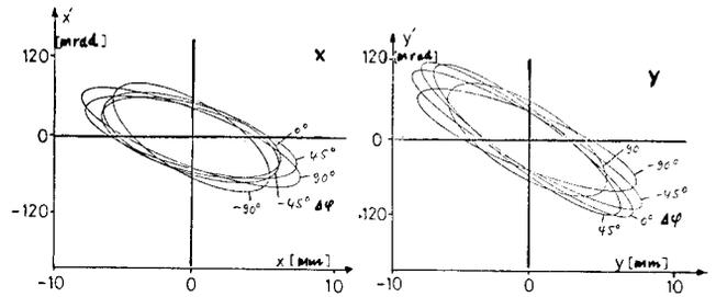
Fig. 8 Transverse acceptances of the MAXILAC-RFQ. Ar<sup>+</sup>-ions, 90 keV,  $\alpha=360$  mm mrad
