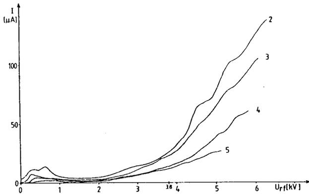
Fig. 7 Transmitted current behind sections 2 - 5 of the proton model as a function of RF voltage
