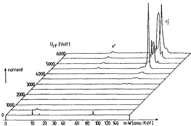
Fig. 3 Energy spectrum behind section 3 of the proton model
