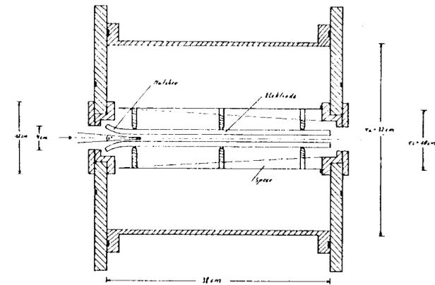
FIG. 10 CROSS SECTION OF SCR FOR HIGH CURRENT BEAM TRANSPORT
