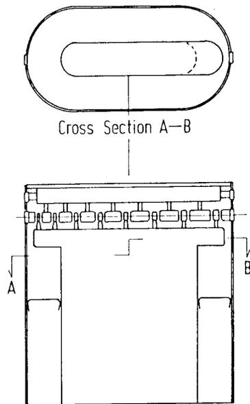
Fig. 1 Concept of a quarter wave coaxial resonator having a race track-type cross section with drift tubes loaded at its open end.
