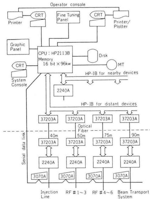
Fig. 6 Block diagram of the control system.
