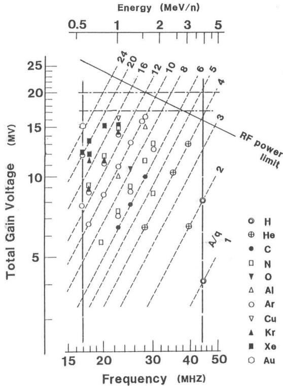
Fig. 9 Distribution of accelerated ions plotted against the frequency and the voltage gain.
