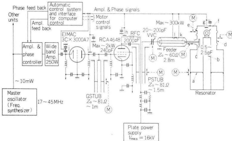
Fig. 4 Frequency tunable high power amplifier circuit.
