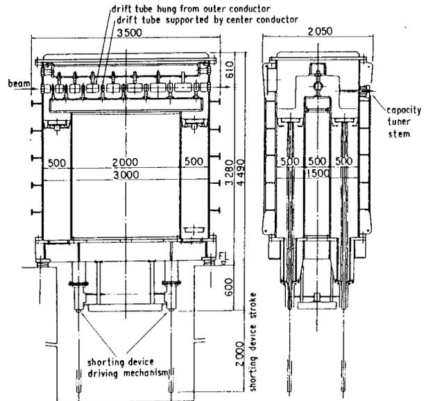
Fig. 2 Engineering design of accelerating structure.
