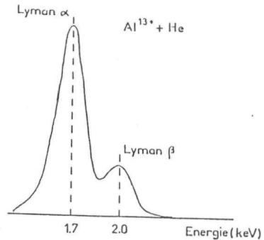
fig.14  $Al^{13+}$  ion beam identified through radiative charge exchange in a Helium target
