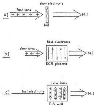
Fig.2. In the foil stripper (a) the ECRIS (b) and the EBIS (c) the same relative collision velocity between the electron and ions with the same  $(nr)$  values give the same charge states of the multicharged ions (M.I.).
