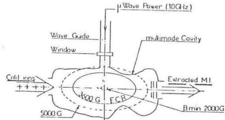
Fig. 3. Main ingredients of an ECRIS-ECR surface in a magnetic well associated with a multimode microwave cavity;
