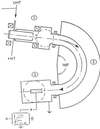
Fig. 9 Ion selection and recording system (1) MINIMAFIOS. (2) Magnetic selector. (3) Collector.
