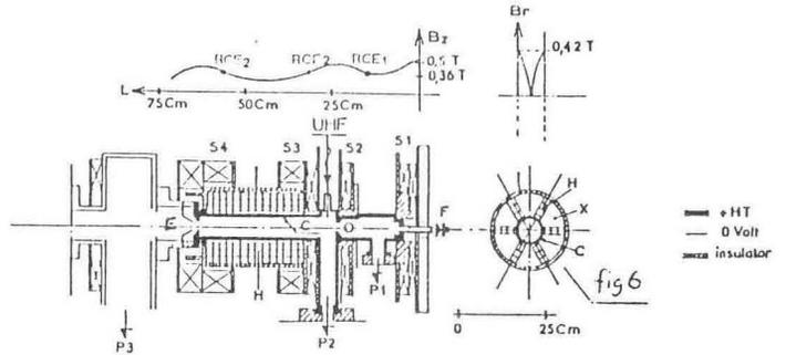
Fig. 5. MINIMAFIOS: F = iron shield; S<sub>1</sub>S<sub>2</sub>S<sub>3</sub>S<sub>4</sub> = solenoids; O = diaphragm; H = SmCo<sub>5</sub> hexapole; I = insulators; [extraction electrode; P<sub>1</sub>P<sub>2</sub>P<sub>3</sub> = pumpings ports; C = multimode cavity; X shield; B<sub>z</sub> = solenoidal magnetic field.
