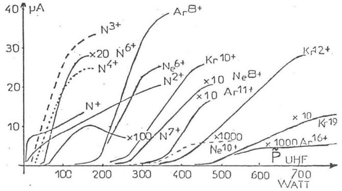
Fig. 10 Ion currents vs. microwave power.
