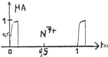
Fig. 11 Nitrogen beam pulses against time.
