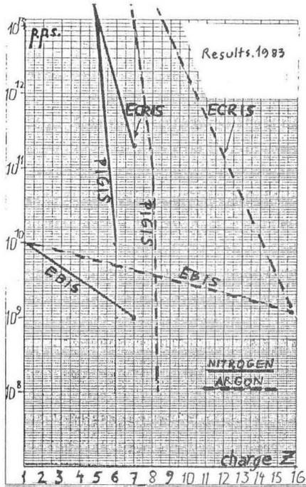
fig.1 Comparative ion yields for Argon and Nitrogen vs charge states (experimental)
