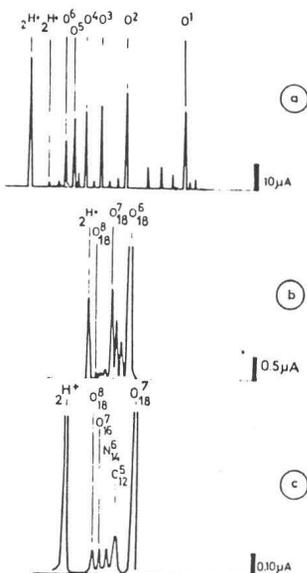
Fig. 13 Charge state spectrum for oxygen: (a) Total spectrum. (b) Enlarged spectrum for highly charged ions. (c) Enlarged spectrum of particles ionized in their K-shell.
