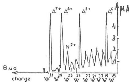
Fig. 15 Typical tungsten ion spectrum  $P = 2$  KW. Duty cycle  $\theta = 0.2$ .
