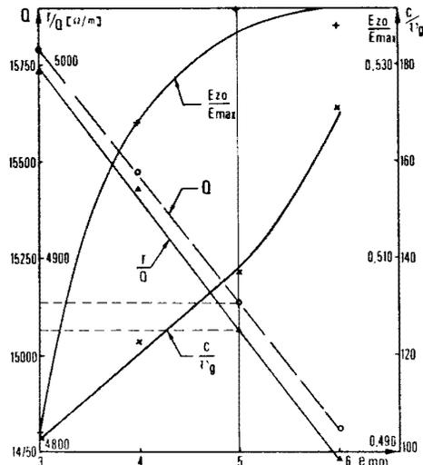
Fig. 2. Cell characteristics versus iris thickness  $e$
