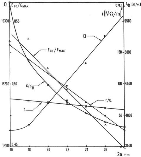
Fig. 3. Cell characteristics versus iris diameter 2a
