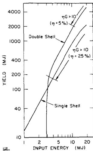
Fig.2 TARGET YIELD vs INPUT ENERGY
