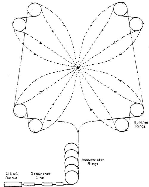
Fig.5 Concept of 4 MJ Driver System at RAL studies by the existing facilities and also accelerator constructions for their purposes are proceeding, as follows.
