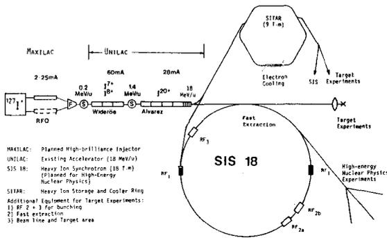
Fig.6 Schematic Layout of SIS-18, SITAR-9 System
