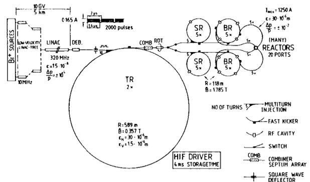
Fig.3 Concept of HIBALL System
