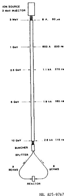
Fig.7 Concept of 3 MJ IL System at LBL<sup>10</sup>
