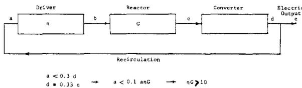
Fig.1 General Scheme of Power Circulation
