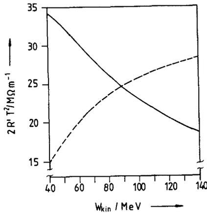
Fig. 4 Shunt resistance of the Alvarez (—) structure, including stems, and the HELA (---) structure;  $2R'T^2$  is the effective shunt resistance per length in the linac style.
