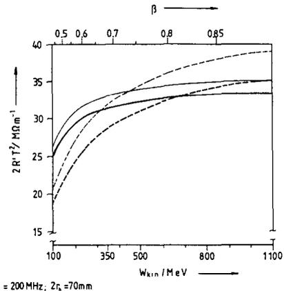
Fig. 5 Calculated Effective Shunt Resistance per Length of
