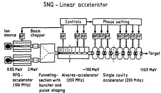
Fig. 1 Schematic illustration of the SNQ rf-accelerator
