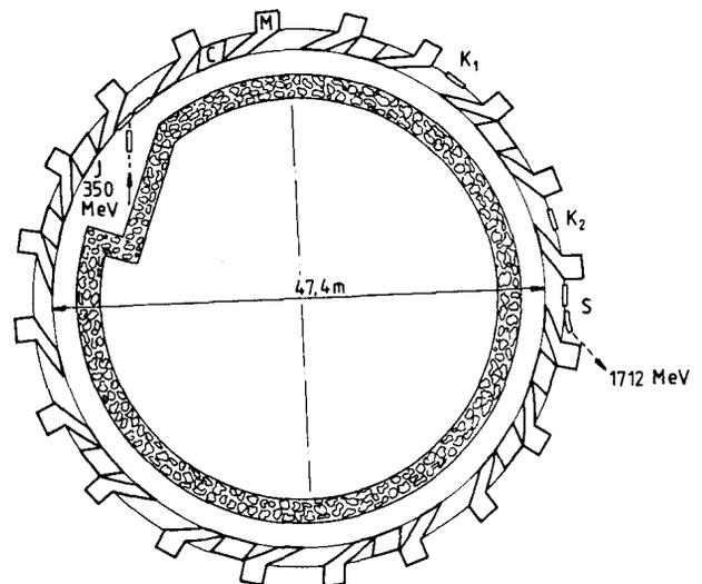
Fig. 9 Schematic layout of an FFAG-compressor
