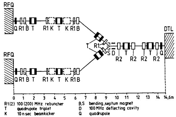
Fig. 3 Concept of the funneling section
