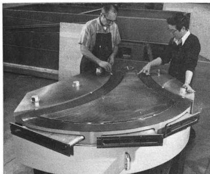
Fig. 10 M7 switching magnet during assembly. Lower yoke, coil, and vacuum chamber are in place.
