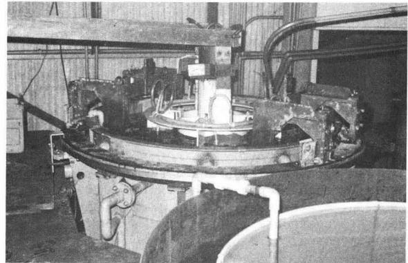
Fig.14 Electroplating bath.
