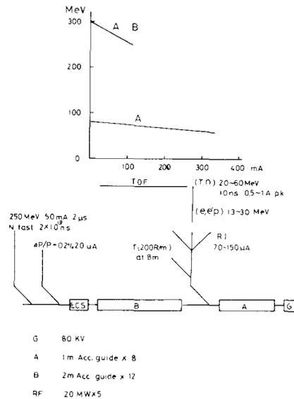
Fig.2 Layout of 300 MeV Tohoku Univ. accelerator.
