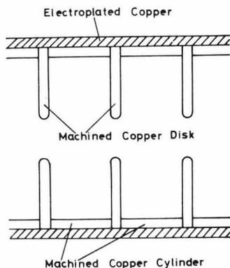
Fig.12(a) Cross section of accelerator guide by means of electro-plating method.
