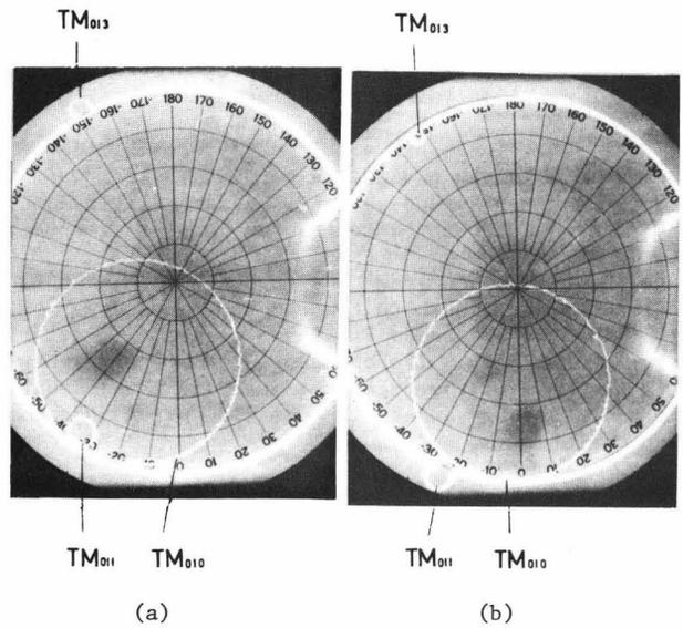
Fig.9 Dynamically balanced impedances looking into two couplers from the respective generators.
