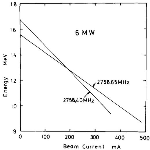
Fig.1 Optimum frequency in heavy loading is different from that of light loading.
