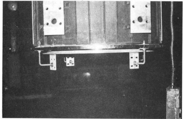
Fig.13 P.V.C. shield attached on a frame of tank to be plated. Suitably shaped nonconducting shield prevents excessive deposition on edges and insures uniform deposits.
