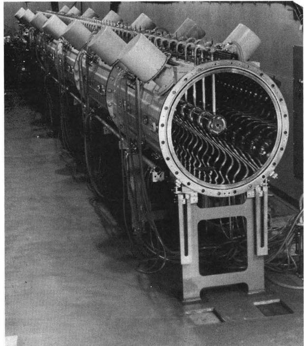
Fig.7 Support of KEK linac tank.
