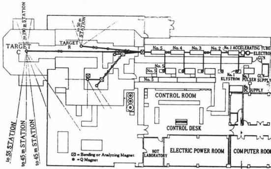
Fig.3 Layout of 150 MeV JAERI accelerator.
