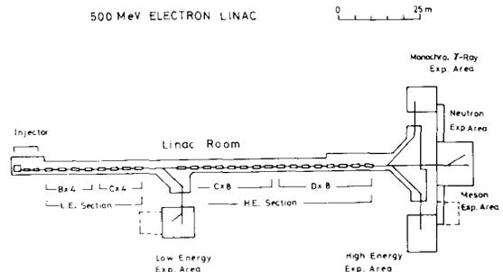
Fig.11 Proposed layout of 500 MeV Electro Tech. Lab. accelerator.
