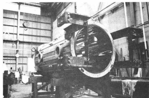
Fig.15 Copper plated unit tank.
