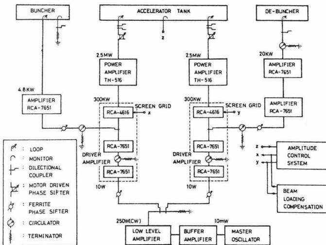
Fig.8 Block diagram of RF system.
