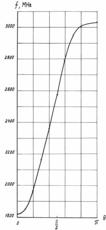
Fig. 3 Dispersion curve of a cavity loaded with washers and discs;  $\beta = 0.8$ ,  $K_c = 47\%$ .
