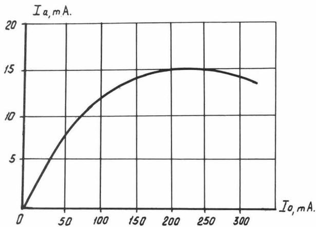
Fig. 5 Limiting current as a function of injected beam current in linac with AAPF.
