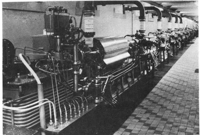
Fig. 7 60 MeV electron linac.
