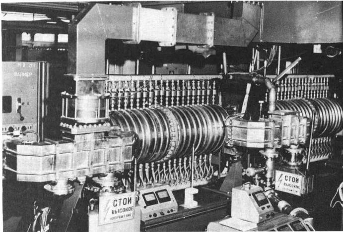
Fig. 1 Prototype resonator for high energy linac section. Structure loaded with washers and discs.
