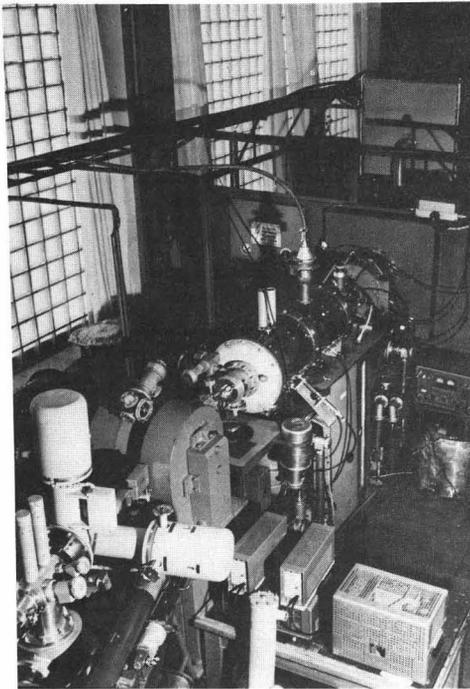
Fig. 6 Experimental linac using the asymmetric alternating phase focusing.
