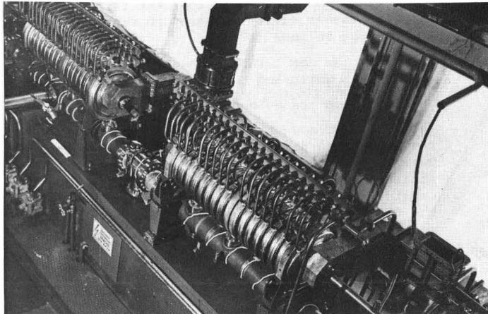
Fig. 2 Prototype resonator for high energy linac section. Ring coupled cells structure.
