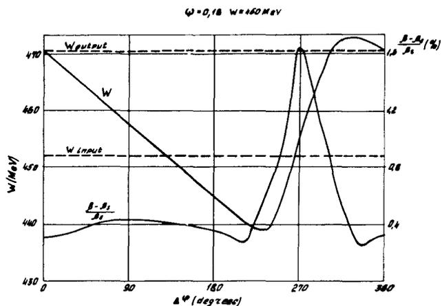
Fig. 4 Energy and velocity spread vs field phase.
