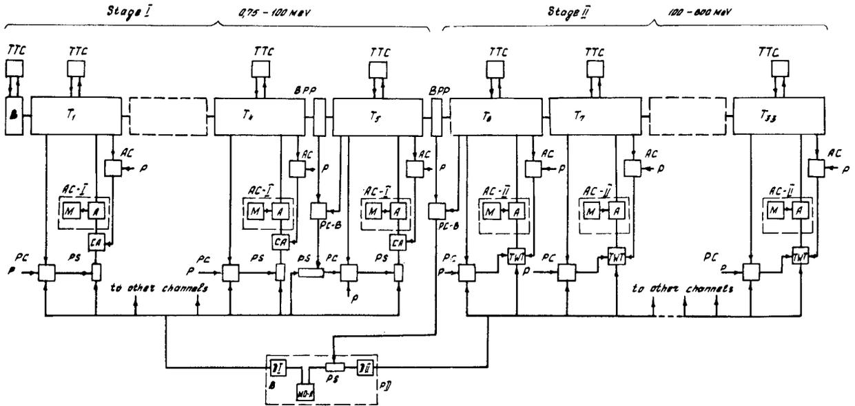
Fig. 9 Simplified block diagram of rf field control system where: B, buncher;  $T_{1-33}$ , tank; M, modulator; A, rf amplifier; AC-I and AC-II, amplifier channels; CA, controlled amplifier; AC, amplitude control; PC, phase
