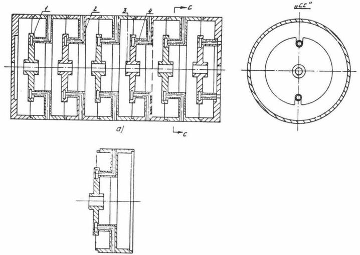
Fig. 6 Accelerating structure loaded with washers and discs
