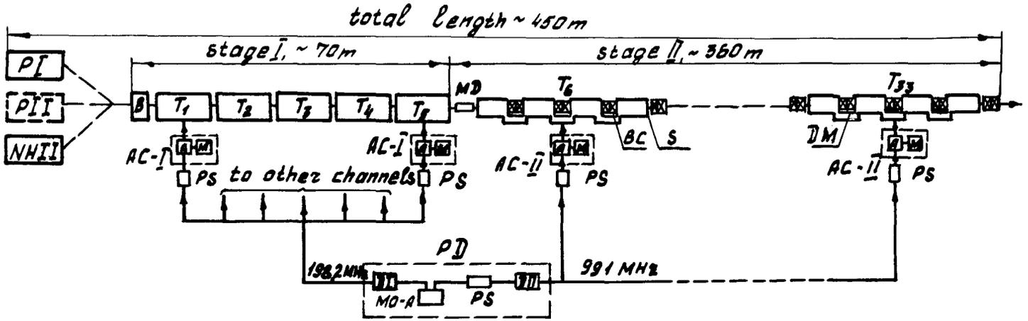
Fig. 1 Block diagram of 600-MeV proton linear accelerator where: PI, proton injector; PII, polarized ion injector; NHII, negative hydrogen ion injector; B, buncher; T<sub>1-33</sub>, tank; MD, matching device;
