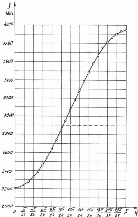
Fig. 7 Dispersion curve of a disc-and-washer loaded structure.
