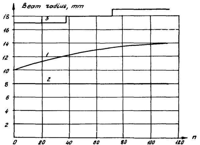
Fig. 3 The beam radius and the beam c.m. displacement as a function of consecutive number of focusing period.
