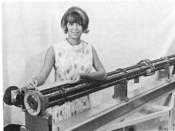
Fig. 12. Typical SLAC microwave technician showing length of troublesome cavities in constant-gradient accelerator section.
