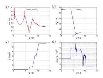
Figure 6: a) transverse trajectories, b) bunch length, c) mean energy, d) relative energy spread in the 100 keV injector.
