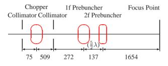
Figure 3: Chopper / prebuncher System (all values in mm).
