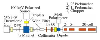
Figure 2: Sketch of the S-DALINAC injector in the accelerator hall.
