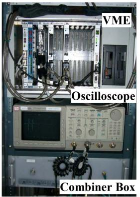
Figure 2: Photograph of a monitor station.
