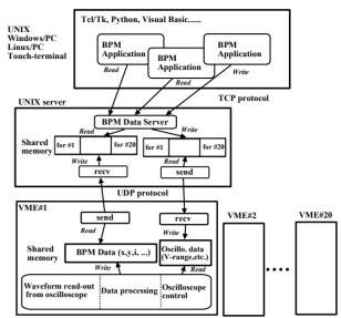
Figure 3: Block diagram of the control software and data flow.
