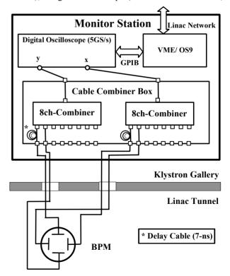
Figure 1: Schematic drawing of a front-end system.
